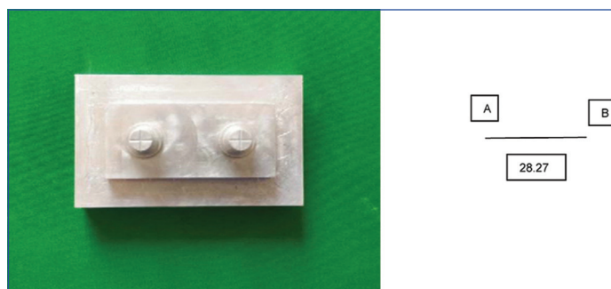
[Table/Fig-2]: Die used for dimensional stability (According to ADA specification no. 19). The dimensions of die with two abutments are labelled as A and B. The diameter of each abutment is 6.330 mm on the occlusal aspect of the abutment, height is 8.015 mm from the finish line to the occlusal aspect of the abutment and distance between the two abutments is 28.270 mm
